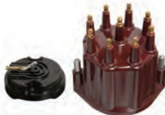
18-5302 TUNE-UP KIT Replaces: Fits: male cap v-8 flamethrower distributors
