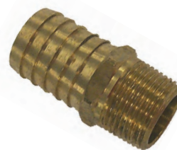
18-4461 HOSE BARB 3/4" - 14 NPT x 1" Hose Corrosion Resistant Brass Fitting
