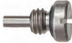
18-2454 DRAIN PLUG 3/8" - 16 thread Replaces: 3854539 For: Volvo SX drives Use o-ring 18-7145
