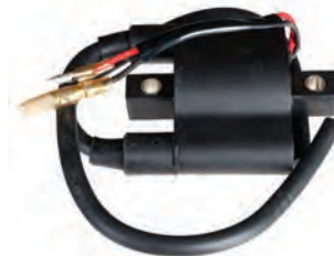
18-5151 IGNITION COIL Replaces: 33410-94400, 33410-92L10 Fits: DT40C(1986-98)
