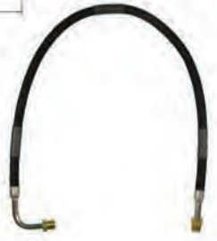
18-8114 FUEL LINE HOSE UNIVERSAL For fuel pump to carburetor connection. Replaces copper or steel tubing 3/8" X 31" PTFE composite hose with 5/8"-18 male inverted flare straight one end, 5/8"-18 90° one end. SAE J1527 type A1
