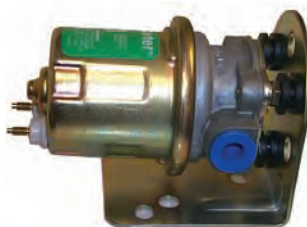
18-7332 ELECTRIC FUEL PUMP Includes bracket and mounting hardware 43 GPH – 7 PSI Max. – 1/4 NPSF for 3/8 hose – operates with both gasoline and diesel fuel - 24 Volt only
