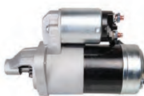
18-6937 STARTER 2 Bolt Flange Replaces: Yanmar 128170-77010, 77010D Hitachi S114-303, 303A Fits: GM, GM2, GM3, GM10, GM20/2- 20F, GM30, GMF, 1GM, 2GM, 3GM
