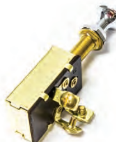
MP39640 MP39642 (Bulk 100pcs./carton) OFF-ON(1)-ON(2) SPDT • First pull energizes #1 • Second pull energizes circuit 2 • Solid brass construction • 3/8" mounting bushing • 3 screw terminals • For panels up to 1" thick • Chrome plated solid brass knob • Rated: 15 amp @ 12 VDC
