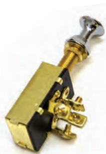
MP39620 MP39622 (Bulk 100pcs./carton) OFF-ON(1)-ON(2&3) SPDT • First pull energizes #1 • Second pull energizes two separate circuits • For anchor/running lights or similar function • Solid brass construction • 3/8" mounting bushing • 4 screw terminals • For panels up to 1" thick • Chrome plated solid brass knob • Rated: 15 amp @ 12 VDC
