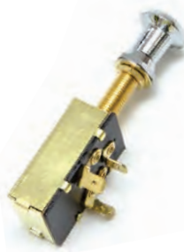
MP39590** MP39592 (Bulk 100pcs./carton) OFF-ON(1)-ON(1&2) SPDT • First pull energizes #1 • Second pull energizes both circuits • Solid brass construction • 3/8" mounting bushing • 3 blade terminals • For panels up to 1" thick • Chrome finish plastic knob • Rated: 15 amp @ 12 VDC
