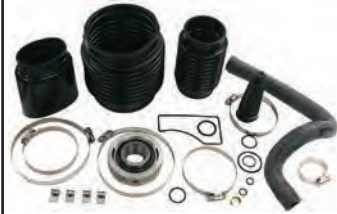
18-8219 TRANSOM SEAL KIT Replaces: 30-803100T1 For: Bravo I/II/III (1988 & Up) S/N 0B664190 & Up; Blackhawk (1994-95) S/N 0F186717 & Up *Sealed Gimbal Bearing 18-21006
