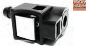
18-80408 FUEL CONNECTOR Replaces: 17650-ZW9-003 Female 5/16" connector with rectangular locking post. Fits late model engine Mates with 18-80407
