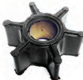
18-3015 IMPELLER Replaces: 396852, 433935, 797407 With Key For: 2.5, 3, 4 Ultra, Excel
