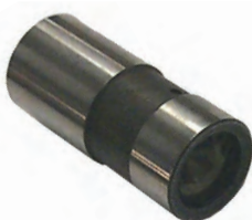
18-1401 HYDRAULIC LIFTER Replaces: 3853847, 985316 Ford 5.0L & 5.8L
