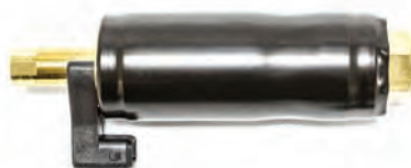
18-7331 ELECTRIC FUEL PUMP • 8 psi, 45 gpm Replaces: OMC/Volvo 3858714, 3850810, 3857985
