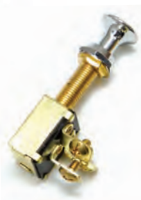
MP39600 MP39602 (Bulk 100pcs./carton) OFF-ON (1 & 2) SPST • Pull for ON - turns on two separate circuits • Solid brass construction • 3/8" mounting bushing • 3 screw terminals • For panels up to 1" thick • Chrome plated solid brass knob • Rated: 15 amp @ 12 VDC
