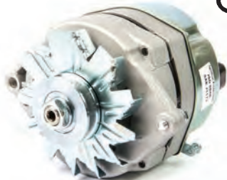
18-5957 ALTERNATOR (3-Wire) (68 amp) Replaces: RA097002, RA097003, RA097006 Replaces Mando, Motorola and original equipment Delco. Uses same electrical connections and mounting method. Equipped with fan and drive pulley. SAEJ1171
