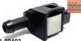
18-80403 FUEL CONNECTOR Female 3/8" hose connector with rectangular locking post, Will not interchange with OE's 5/16" hose assemblies. For late model engine: For use with our 18-81042 fuel hose assembly, motor end. Mates with 18-80407
