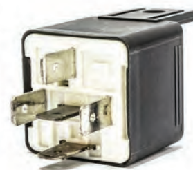
18-6266 RELAY Replaces: 876040, 872300 12 Volt, 30 Amp/20 Amp continuous
