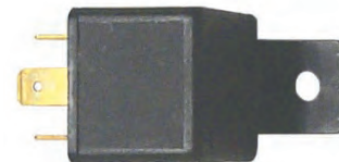
18-5704 POWER TRIM RELAY Replaces: 876037 20 Amps Resistive 15 Amps Inductive Single Pull 5 Terminal For: AQ270, 280
