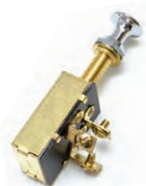
MP39580** MP39582 (Bulk 100pcs./carton) OFF-ON(1)-ON(1&2) SPDT • First pull energizes #1 • Second pull energizes both circuits • Solid brass construction • 3/8" mounting bushing • 3 screw terminals • For panels up to 1" thick • Chrome plated solid brass knob • Rated: 15 amp @ 12 VDC
